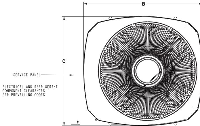
TOP DISCHARGE AREA SHOULD BE UNRESTRICTED FOR AT LEAST 1524 (5 FEET) ABOVE UNIT. UNIT SHOULD BE PLACED SO ROOF RUN-OFF WATER DOES NOT POUR DIRECTLY ON UNIT, AND SHOULD BE AT LEAST 305 (12") FROM WALL AND ALL SURROUNDING SHRUBBERY ON TWO SIDES. OTHER TWO SIDES UNRESTRICTED.
